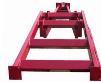
Heavy duty tubular frame with 6500 lbs tandem Henschen Axles
