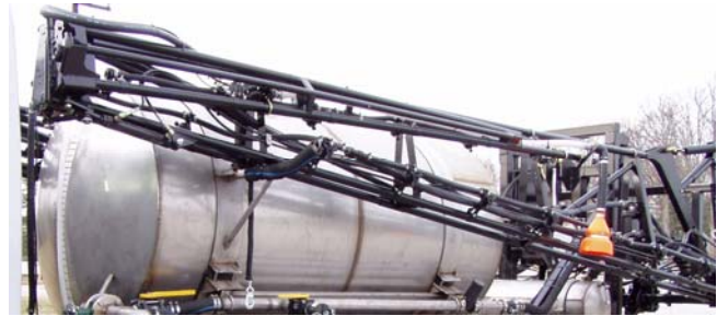
60 Foot Tubular Construction Booms With Hydraulic Tip Fold Breakaways
