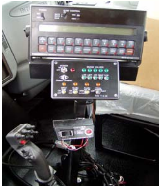
Electronic Flow Controls With Boom Switchbox And Joystick Boom Control
