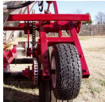
Hydraulically operated press wheel w/ easy switch from fertilizer to lime.
