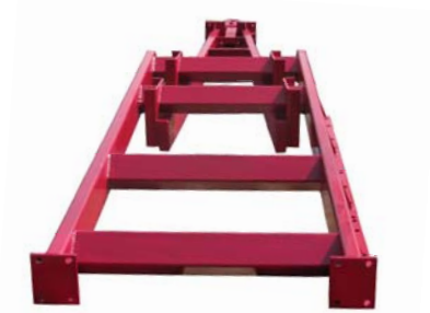
Heavy duty tubular frame with 6500 lbs tandem Henschen Axles
