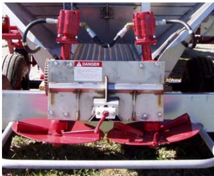
Top mounted hydraulic motors with 24" spinner plates and stainless steel back plate and bumper
