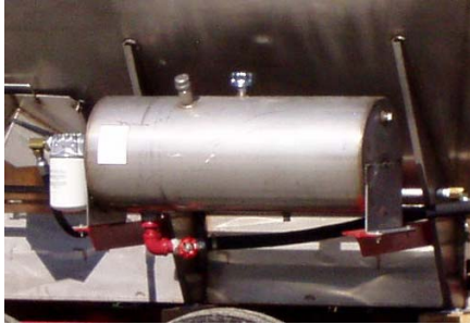
Large capacity stainless steel hydraulic oil tank w/ shut off valve and return filter
