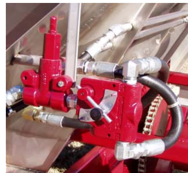
Hydraulic controls for spinner speed control and pressure relief
