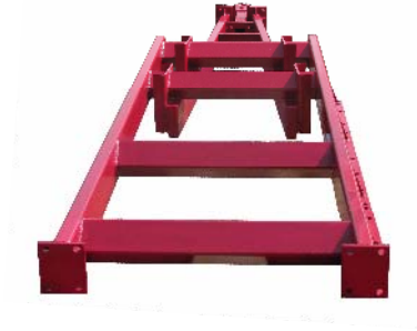
Heavy duty tubular frame with 6500 lbs tandem Henschen Axles
